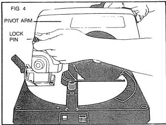
To release the pivot arm, remove the cardboard filler block and grasp the switch handle with one hand and the end of the lock pin with the other, as shown in Fig. 5. (the cardboard filler block you removed contains the wing knob.) Push down on the switch handle lightly and pull out on lock pin. When the pin is out as far as it will go, raise the pivot arm to its full height. (The saw will look like the picture on the front cover of this manual.)
