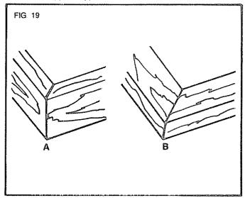
The example in Fig. A is a joint made by using the bevel adjustment to bevel the edges of the boards (at 45° each) to form a 90° miter corner. For this operation, set the bevel post adjustment of 45° and the miter table adjustment at 0°. Position the wood with the broad flat side against the table and the narrow edge against the fence.
