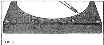
5. When you have set the desired angle, lock it in place by tightening the two miter clamp knobs that you loosened in Step 2 above.
