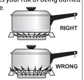
**For most cooking**, start on the highest control setting and then turn to a lower one to complete the process. Use the chart below as a guide for determining proper flame size for various types of cooking. The size and type of utensil used and the amount of food being cooked will influence the setting needed for cooking.
