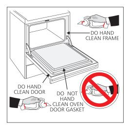
door open. This can damage the automatic door locking system. Use caution when opening the door after the self-cleaning cycle is completed. The oven may still be VERY HOT.
