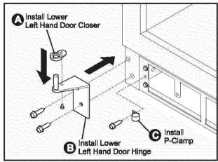
14 Remove button plug from upper left side of door and place in upper right side of door. Place door on lower LH hinge bracket.
