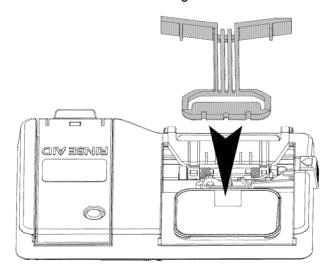
• Press into place, to seat the water diverter.
