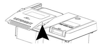
• Slide the bottom of the door guides off the track of the module.
