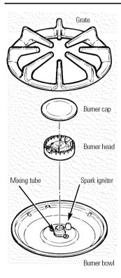
**CAUTION:** DO NOT OPERATE THE BURNER WITHOUT ALL BURNER PARTS IN PLACE.
