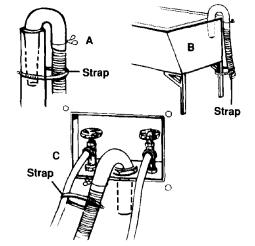
Put "hook" end of drain hose in tub or standpipe. Tightly wrap the shipping strap around the drain hose and tub or standpipe or inlet hose as shown in Figures A-C. Push plug into the nearest hole in the shiping strap. Untape power supply cord and plug into grounded outlet.
