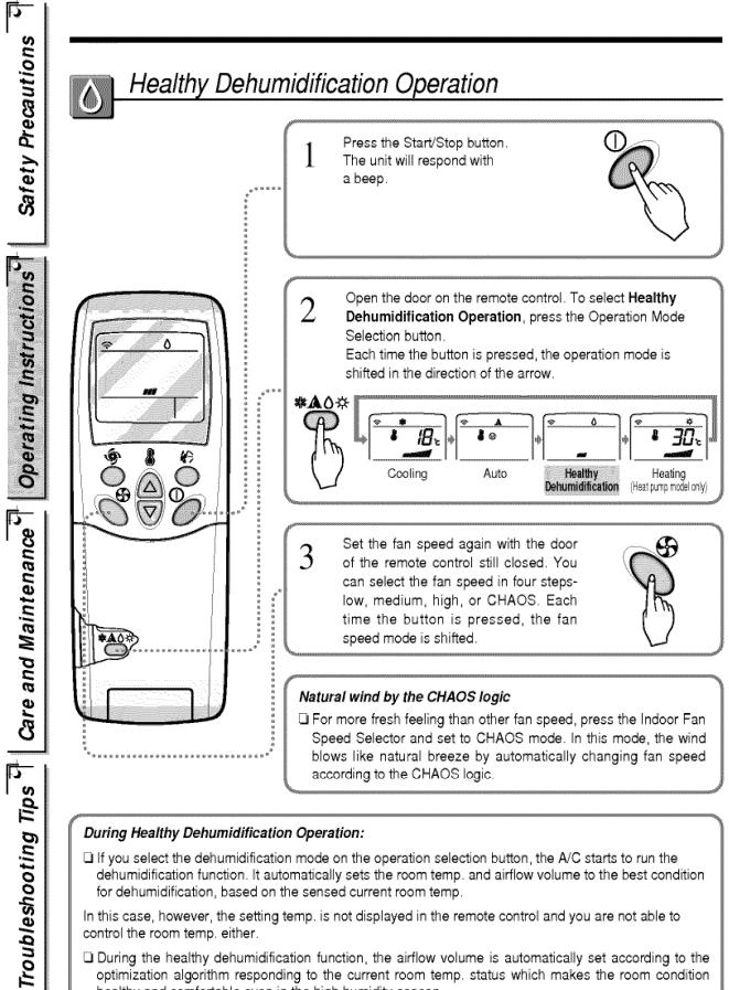
If you select the dehumidification mode on the operation selection button, the A/C starts to run the dehumidification function. It automatically sets the room temp. and airflow volume to the best condition for dehumidification, based on the sensed current room temp.
