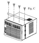
NOTE: FOR SAFETY REASONS, ALL FOUR (4) SCREWS <u>MUST</u> BE SECURELY FASTENED.
