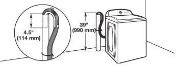
Minimum diameter for a standpipe drain: 2" (51 mm). Minimum carry-away capacity: 17 gal. (64 L) per minute. Top of standpipe must be at least 39" (990 mm) high; install no higher than 96" (2.44 m) from bottom of washer. If you must install higher than 96" (2.44 m), you will need a sump pump system.
