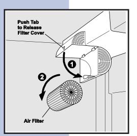
The air filter is located on the back of the control box. In general, you should change the air filter every six months to ensure optimal filtering of refrigerator odors. You may want to adjust this time period depending on the types and amounts of food you typically store in your refrigerator.
