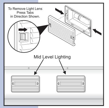
the lamp housing by unsnapping it from the lamp housing using your fingers or a screwdriver. Be careful not to break the locking tabs on the lamp housing. Replace the old bulb with a bulb of the same type and wattage. To replace the lens, snap one side of the lens opening to the tab on the lamp housing. Then carefully attach the other side.
