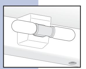
The light comes on automatically when the door is opened. The light bulb assembly is located on the back of the freezer control box. To replace the light bulb, turn the temperature control to "OFF" and unplug the electrical cord. Replace the old bulb with a bulb of the same type and wattage.
