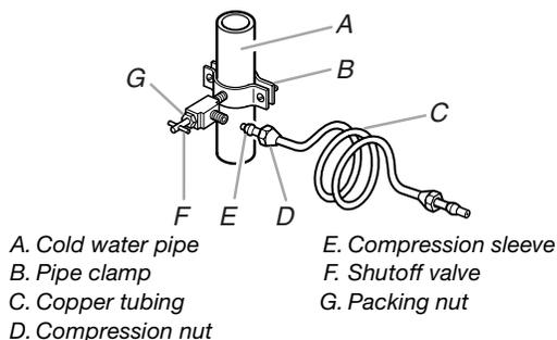
6. Fasten the shutoff valve to the cold water pipe with the pipe clamp. Be sure the outlet end is solidly in the ¼" (6.35 mm) drilled hole in the water pipe and that the washer is under the pipe clamp. Tighten the packing nut. Tighten the pipe clamp screws slowly and evenly so the washer makes a watertight seal. Do not overtighten or you may crush the copper tubing.
