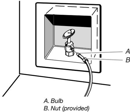
4. Turn shutoff valve ON.
