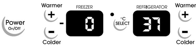
To turn the refrigerator on, press and hold POWER (ON/OFF) for 2 seconds. The factory recommended set points are 0°F (-18°C) for the freezer and 37°F (3°C) for the refrigerator.
