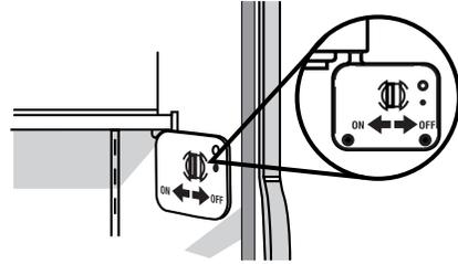
To turn on the ice maker, slide the control to the ON (left) position.
