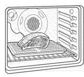
The temperature probe has a skewer-like probe at one end and a plug at the other end that goes into the outlet in the oven. Use of probes other than the one provided with this product may result in damage to the probe.
