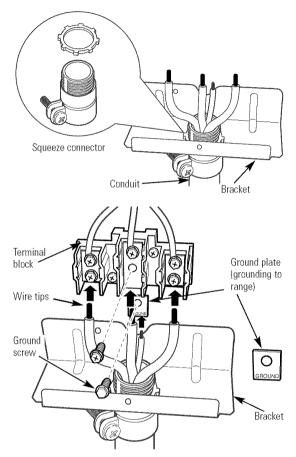
Wire used, location and enclosure of splices, etc., must conform to good wiring practices and local codes.
