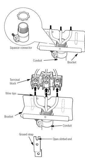
Wire used, location and enclosure of splices, etc., must conform to good wiring practices and local codes.
