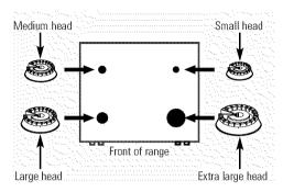
Make sure the slot in the burner head is positioned over the electrode.
