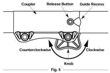
**NOTE:** Aligning the release button with the guide recess will help installation (Fig. 5).
