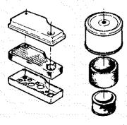
Generally, wash foam-type filters in a dishwashing detergent and water solution. Rinse and wring dry, then saturate with oil and squeeze out excess. Failure to re-oil this type filter will ruin the engine.
