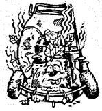
Air is also needed to keep your engine cool. Dirt, dust & debris build up restricts and clogs cooling air intake screens and fins. Clean screens and fins at frequent intervals. The engine blower housing and shrouds should be removed at least once each season or more often under dry, dusty conditions for a thorough cleaning of fins.
