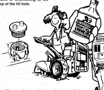
Change oil at regular intervals using a high quality oil such as Snapper's small engine formulated 4-cycle engine oil. Refer to the engine owner's manual for oil details.
