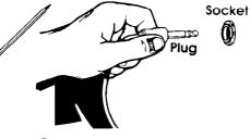
2. Place food in the oven and plug the probe plug into the socket on the back oven wall.
