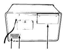
**3.** Do not block the vent or air intake openings on the rear of the oven. Blocking vent or air intake openings can cause damage to the oven and poor cooking results. Make sure the microwave oven legs are in place to ensure proper air flow.
