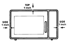
**4.** Do not install the microwave oven so that both sides and the top are flush with walls, shelves or cabinets. Both sides and the top must have at least 1 in. (2.54 cm) clearance for proper operation.
