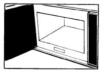
**NEVER** start a microwave oven when it's empty. The oven can be damaged. If you experiment, put a container of water in the oven.
