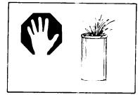
WARNING – Use care when heating liquids or adding ingredients to heated liquids. Liquids heated in certain shaped containers may become overheated. The liquid may splash out with a loud noise during or after heating or when addIng ingredients (instant coffee, etc.). This can harm the oven and the hot liquid could burn you. Do not use such containers to heat liquids again.
