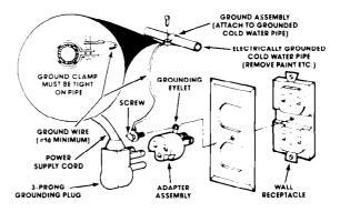
If changing and properly grounding the wall receptacle is impossible and where local codes permit (consult your electrical inspector), a temporary adapter may be plugged into the existing 2-prong wall receptacle to mate with the 3-prong power supply cord. THIS, HOWEVER, IS NOT RECOMMENDED.
