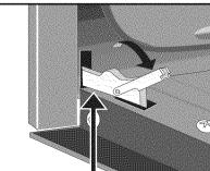
Lock engaged for door removal
