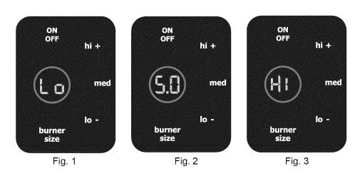
The **hi+** and **lo-**keys provide incremental adjustments for more precise control when changing settings between the lower heat levels (Lo to 3.0 power levels). Higher heat level setting changes (between 3.0 to HI) will change much faster.
