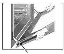
HINGE SLOT - Door removed from the appliance
