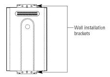
4 ON WOOD OR SIDING: When attaching the unit to wood or siding, mount 2 boards suitable for anchoring to wall studs, between the studs. You can do this before the wall has been finished.
