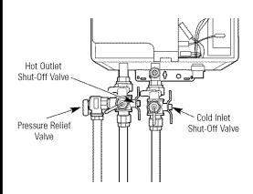
Water connections to the tankless water heater should follow all state and local plumbing codes.
