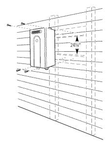
NOTE: Screws provided must fasten securely and directly into wood. If screws go through siding or insulation and do not fully engage, installer must supply correct screws.
