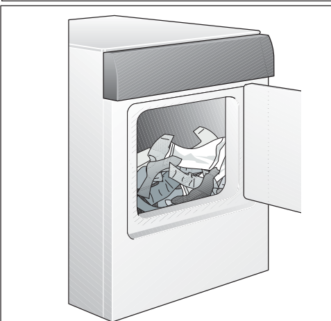
Fill dryer drum 1/3 to 1/2 full.
