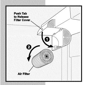
The air filter is located on the back of the control box. In general, you should change the air filter every six months to ensure optimal filtering of refrigerator odors. You may want to adjust this time period depending on the types and amounts of food you typically store in your refrigerator.
