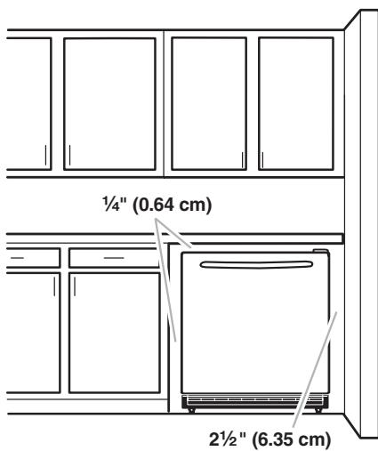
To ensure proper ventilation for your refrigerator, allow for a  $\frac{1}{4}$ " (0.64 cm) space on each side and at the top. When installing your refrigerator next to a fixed wall, leave  $2\frac{1}{2}$ " (6.35 cm) minimum clearance on each side to allow for the door to swing open.
