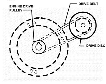
TOP VIEW OF STRETCH TYPE BELT ROUTING
