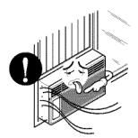
Do not use the power cord near flammable gas or combustibles such as gasoline, benzene, thinner, etc.
