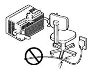
Turn off the power and breaker firstly when cleansing the unit.
