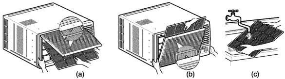
**NOTICE** : Mark  $\Delta$  of inlet grille means opening direction.
