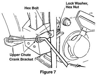
• Place the hex bolt into the hole provided in the left handle. Fasten with lock washer and 5/16 hex nut from the same group of the hardware pack. Do not tighten until after attaching the other end of the chute crank.
