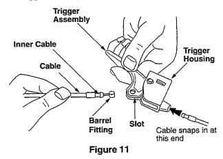
**Note:** When the cable is installed correctly, you should not be able to pull the cable out of the trigger housing.
