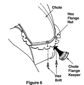
After assembling all three chute flange keepers, tighten, then back off 1/4 turn to allow easier movement of the chute. Use (2) 7/16" wrenches.
