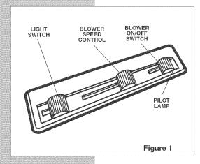
The blower on/off switch turns the blower on to the running speed set by the blower speed control. The blower must be turned on and off using this switch.
