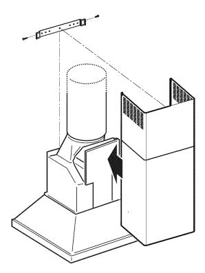
• Secure the bottom of the duct with 2 assembly screws provided.
