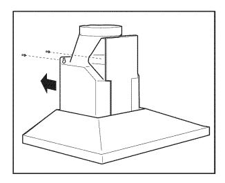
Mark "lower" wood screw holes locations in the wall using a pencil.
