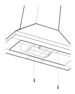
Instal the grease filter and turn power on at service panel. Check operation of the hood.
