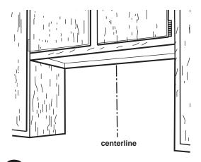
Determine and clearly mark a vertical centerline on the wall and cabinet in the area the vent opening will be made.
