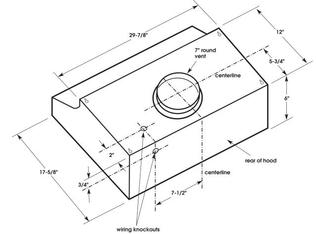
A 115-volt, 60-Hz, AC-only, fused electrical supply is required. The total ampere load used, including the range hood, must not exceed 90% of the rated capacity of the circuit. The ampere rating of the range hood is located on the model/serial number rating plate located on the side cover of the fan motor housing.
