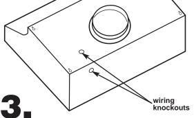
Remove knockout from the wiring opening (top or rear) to be used.
