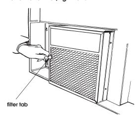
Pull firmly on filter tab to remove filter/light lens from range hood..
