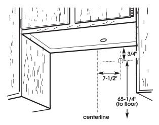
**To wire through rear**, mark a line 7-1/2" from the right of the centerline on the wall. Mark the point on this line that is 65-1/4" from the floor (or 3/4" from underside of cabinet). Drill a 1-1/4" diameter hole through wall at this point.
