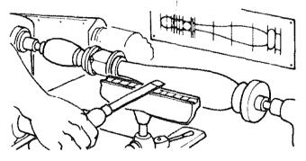
Using a Template and a Diameter Board
