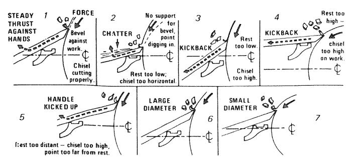
If the rest is placed too low, so that the chisel is held with the bevel out from the work (sketch 2), the cutting edge will continue to dig deeper into the work. It will dig in until the "bite" becomes so deep that your hands have difficulty holding the chisel — then the improperly supported chisel will begin to bounce, or chatter, against the workpiece.
