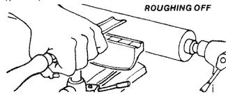
Roughing-off and other heavy work requires a firm grip and solid positioning of the chisel against the rest. This is best
