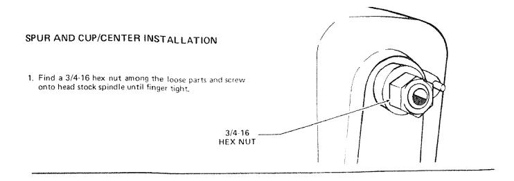
2. Find two points and a spur and cup center among the loose parts. To insert point into centers, place center between jaws of a vise. Do not tighten vice. Insert point into center and with a hammer and nail gently tap around the base of the point until secure.
