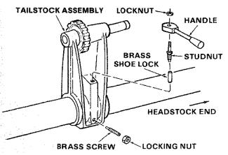
Install the rear foot onto the tube as shown and tighten rear foot locking screw. Foot will wedge into place as screw is tightened. This may take several attempts.
