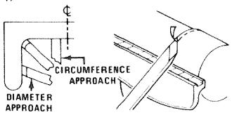
Either a cutting or scraping action can be used when the approach is toward a circumference — the shaving is removed like a peeling from a potato. Scraping, only, can be used when the approach is toward a diameter. The reason is obvious when you consider that faceplate turning practically always requires removal of wood across the grain. Wood does not peel easily across the grain, and attempts to use cutting methods will likely result in damage to the work and throwing of the chisel by the work.
