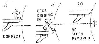
does the scraping, sketches 9 and 10 show the results of too low or too high a position for the rest; and sketch 8 shows the chisel action with the rest correctly positioned.
