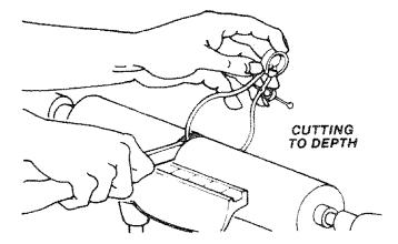
Many scraping operations and cutting to depth with the parting tool can be done with one hand. The chisel is grasped firmly, with the index finger on top to press it down against the rest — and is thrust straight into the work. Holding the tool thus leaves the other hand free to hold a pattern, calibers, etc., to check work progress.
