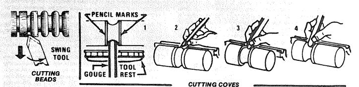
From this start, depress point slightly to start cut, then continue to move point down in an arc toward the bottom center of cove - at the same time rolling chisel uniformly so that, at the end of the cut, it will be flat at bottom of the cove. The object is to keep the extreme point of gouge doing the cutting from start to finish. Reverse movements to cut the opposite side.
