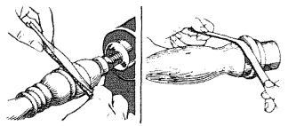
Turnings should be sanded with the lathe running in second lowest speed. A large sheet of sandpaper is useful for smoothing cylinders. All other sanding operations are done with a narrow strip of abrasive paper. The best finishing grit is 3/0 for softwoods, 4/0 for hardwoods.
