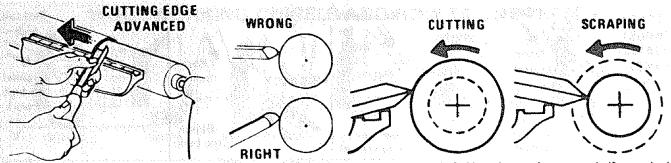
When used for cutting, the gouge is always held with the convex side down. It should be rolled approximately 30° to 45° in the direction in which it is being advanced along the rest; and the cutting edge should be a little in advance of the handle.
