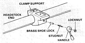
5. Attach the tool rest holder to the clamp support as shown.
