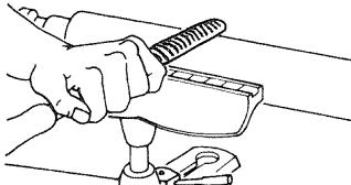
Finer finishes (similar to those produced by scraping) can be obtained by using files in the same manner. Various shape files can be used for shaping vees, beads, coves, etc. If pressed into the wood too hard, however, a file can burn the workpiece surface. Keep the file clean to keep it cutting uniformly. Files work best on hardwoods.
