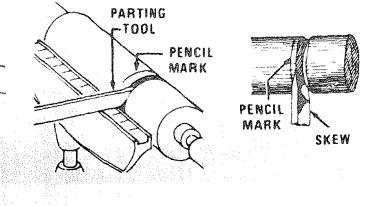
First, mark position of the shoulder with a pencil held to the revolving workpiece. Then make a sizing cut with the parting tool, placing this cut about 1/16-in. outside the shoulder position, and cutting to within about 1/8-in. of the depth desired for the area outside of the shoulder. If shoulder is shallow, the toe of the skew can be used to make the sizing cut; but do not go in deeper than 1/8-in. with the skew unless wider and wider vees are cut to provide clearance for this tool.
