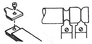
The holder should provide a shoulder against which the butt end of the knife can be firmly seated; and the knife must be securely mounted, either by means of a screw threaded into the holder, or by compressing it between two prongs bolted together.
