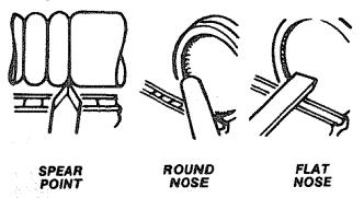
The spear point is used for fine scraping and delicate operations, such as the forming of beads, parallel grooves and shallow vees. Edges and bowl contours can be rounded with the round nose chisel. Any flat surface can be scraped with the flatnose chisel.
