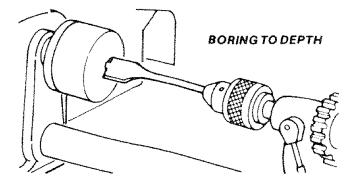
Now remove the bulk of the waste (to rough-out the desired recess) by scraping with the roundnose chisel or the gouge. Remove up to within 1 /8-in. of finished size in this manner. Finish off the inside circumference by scraping with the spear-point chisel or skew. Smooth the bottom of the recess by scraping it flat with the flatnose chisel.
