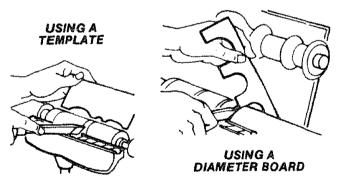
If a great many turnings are being produced, a diameter board will save the time used for resetting calipers. This is simply a thin board along the edge of which a number of semi-circular cuts have been prepared to represent all the various caliper settings required for measuring the sizing cuts. Each semi-circular cut is held against the workpiece instead of using the calipers.
