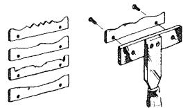
When a number of identical pieces are to be produced, all having a distinctive surface pattern, preformed tools will speed the work and assure uniformity. Patterns like those illustrated can be created by grinding thin (.020 to .010) gauge aluminum strips. A holder, like the one shown, can then be used to support any one of your prepared strips —and guide it against the workpiece.
