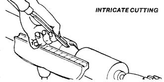
Intricate, delicate cutting requires extreme control, with practically no force. This is best accomplished by guiding the chisel with the fingers of the tool-rest hand. The hand is held palm up, with the wrist high — with the little finger placed against the rest to steady the hand. The chisel does not touch the rest; and the handle hand is completely secondary to the tool-rest hand.
