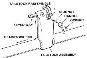
8. On the backside of the tailstock assemble the locking devices as shown.
