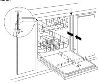
• Fasten the dishwasher to the underside of the countertop with the 2 Phillips screws provided.
