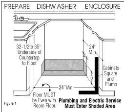
The rough cabinet opening must be at least 24"deep and 23-5/8"To 24" Wide. The opening should be to 35"max, height.  The dishwasher must be installed so that drain hose is no more than 10 feet in length for proper drainage.
