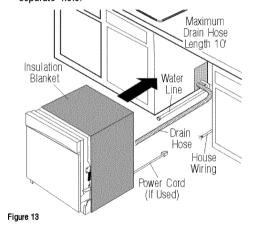
**TIP:** Position water line and house wiring on the floor to avoid interference with base of dishwasher.
