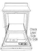
Level the dishwasher by adjusting the four leveling legs individually.
