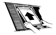
2. Slide the griddle into place with drain slot at rear.
