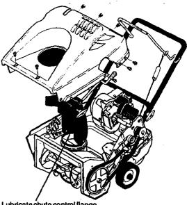
Lubricate chute control flange. Coat flange with a clinging type grease such as Lubriplate.
