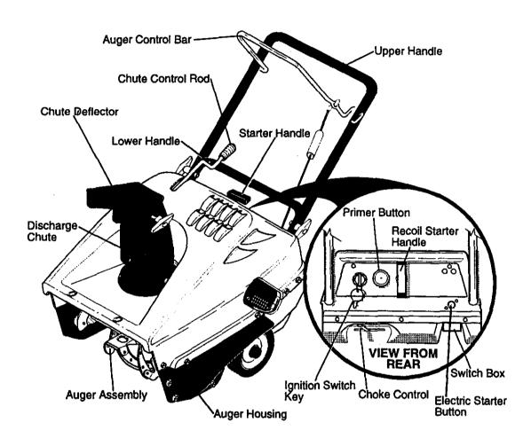
Auger Control Bar – Starts and stops the auger which propels the snow thrower.
