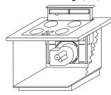
**Note:** Telescopic downdraft vents are not recommended to be installed with cooktops that are flush mounted.
