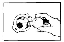
2. Remove the light bulb from its socket. Replace with a 40-watt appliance bulb. Plug in appliance or reconnect at the main power supply.
