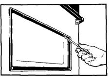
1. Turn off all controls. With the door closed, remove the screws from the top of the outer window frame.
