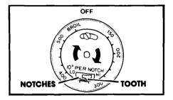
**4. To raise the temperature,** move the tooth a notch closer to HI. Each notch equals about 10°F (5°C).
