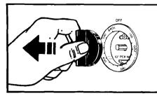
**1.** Pull the Oven Temperature Control Knob straight off.
