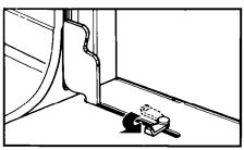
3. Rotate the Broil Stop clips over the door hinge slots and close the door to the Broil Stop position (open about 4 inches, 10.2 cm). The door will stay open by itself.
