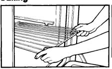
The rack(s) should be placed so the top of the food will be centered in the oven. Always leave at least 1½ to 2 inches (4-5 cm) between the sides of the pan and the oven walls and other pans. For more information, see the Cooking Guide.
