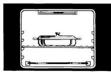
**4.** Put food in the oven. During baking, the elements will turn on and off to keep the oven temperature at the setting. The Oven Indicator Light will turn on and off with the elements.
