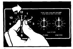
Let the Minute Timer Knob pop out. Turn clockwise until Minute Timer hand points to OFF. The clock setting will change if you push in the knob when turning.
