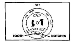
**3.** To lower the temperature, move the tooth a notch closer to LO. Each notch equals about 10°F (5°C).
