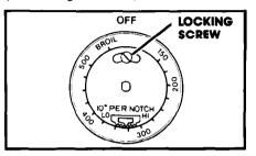
2. Loosen the locking screw. Note the position of the notches.
