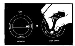
3. Set the Oven Temperature Control to the baking temperature you want. The Oven Indicator Light will come on. The oven is pre-heated when the Oven Indicator Light first goes off.
