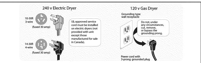
Avoid fire hazard or electrical shock. Do not use an adaptor plug or extension cord or remove grounding prong from electrical power cord. Failure to follow this warning can cause serious injury, fire or death.
