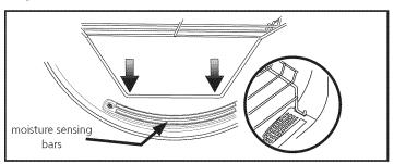
Place items to be dried on top of the rack, leaving space between items and not allowing them to hang over the sides or through the holes. The weight should not exceed 10 lbs (4.5 kg). Select the air (no heat) setting for items containing plastic, foam rubber, rubber-like materials, feathers or down.
