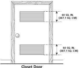
5. The following illustrations show minimum clearance dimensions and air openings for proper operation in a recess or closet installation.
