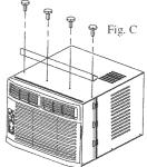
NOTE: FOR SAFETY REASONS, ALL FOUR (4) SCREWS <u>MUST</u> BE SECURELY FASTENED.
