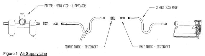
Always disconnect tool from air supply when servicing or adjusting tool and when tool is not in use.
