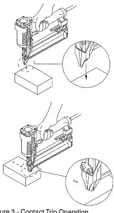
Figure 3 - Contact Trip Operation
