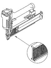
Figure 2 - Loading Finish Nails
