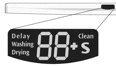
The WASHING light comes on at the beginning of cycle and remains on until the end of the main wash.
