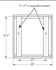
The support must be level and rigidly mounted, flush with the bottom edge of the cutout.
