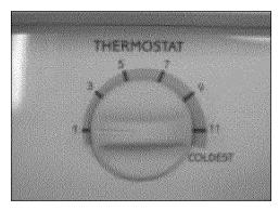
When a COOL or HEAT (some models) setting is selected, the thermostat controls the amount of cooling or heating by automatically turning the cooling compressor or heater on and off in response to the room temperature.
