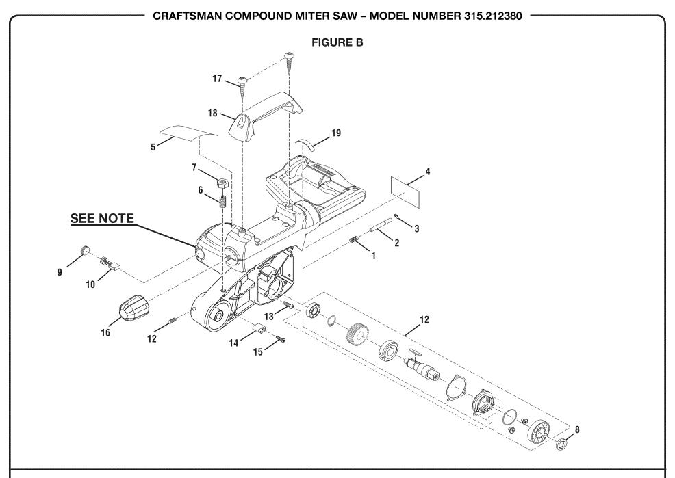
**NOTE:** The assembly shown represents an important part of the double insulated system. To avoid the possibility of alteration or damage to the system, service should be performed by your nearest Sears Repair Center. Contact your nearest Sears retail store for service center information.
