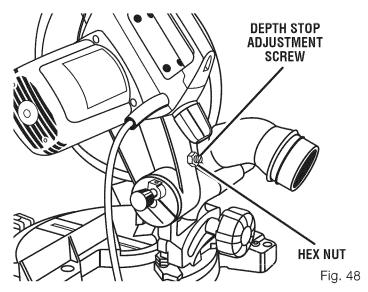
**CAUTION:** Do not start the compound miter saw without checking for interference between the blade and the throat plate. Damage could result to the blade if it strikes the throat plate during operation of the saw.
