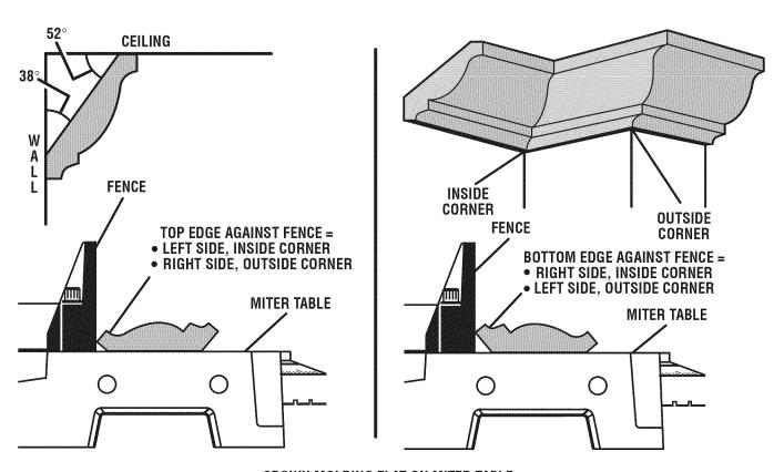
**CROWN MOLDING FLAT ON MITER TABLE**
