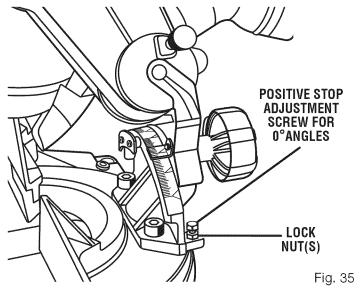
This saw has two scale indicators, one on the bevel scale and one on the miter scale. After squaring adjustments have been made, it may be necessary to loosen the indicator screws and reset them to zero.
