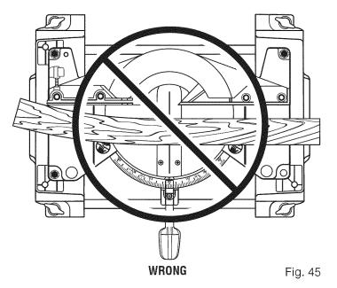
**WARNING:** To avoid a kickback and to avoid serious personal injury, never position the concave edge of bowed or warped material against the fence.
