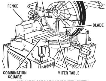
VIEW OF BLADE NOT SQUARE WITH MITER TABLE, ADJUSTMENTS ARE REQUIRED Fig. 34
