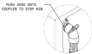
3. Using pliers, squeeze the ears of the spring clamp and position the clamp so the clamp ears <u>align with</u> <u>and contact the tabs</u> on the drain hose. This assures proper location of the clamp to prevent leaks.
