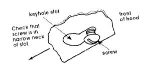
Lift range hood into final position, feeding electrical wire through wiring opening. Tighten mounting screws to cabinet, making sure mounting screws are in narrow neck of slot.
