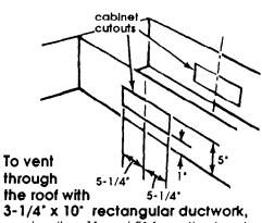
3-1/4' x 10' rectangular ductwork, mark a line 1' and 5' from the back wall on the underside of the cabinet. Mark lines 5-1/4' to the right and left of the centerline on the underside of cabinet that connect the lines just drawn. Use a saber saw to cut a rectangular opening for the ductwork. Repeat for the underside of the top of the cabinet.
