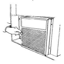
Pull firmly on tab to remove filter/light lens from range hood.
