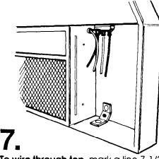
To wire through top, mark a line 7-1/2" from the right of the centerline on the underside of the cabinet. Mark the point on this line that is 1-3/8" from the back wall. Drill a 1-1/4" diameter hole through cabinet at this point.
