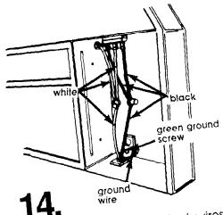
Connect the white and black wires of the power supply cable to the white and black leads in the hood with twist-on connectors.
