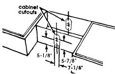
To vent through the roof with 7" round ductwork, mark 5-1/8' and 5-7/8' in from back wall along the centerline on underside of cabinet. Use these points as centers to draw 7-1/8' circles on underside of cabinet.
