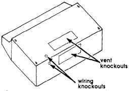
Remove knockout from the wiring opening (top or rear) to be used.
