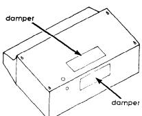
10. If roof or wall cap does not have a damper, attach rectangular damper supplied with hood to selected rectangular vent opening. If damper is attached to back of range hood, be sure damper hinge is toward the top.
