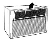
Grab the tabs on the filter and pull it up and out.
