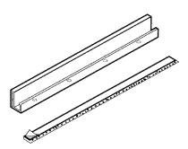
Install the top mounting rail with 4 type A or 5 type A screws (as the installation requires) from the outside of the case.
