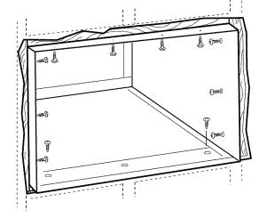
Place the case in the wall opening and secure with 12 1" long #10 wood screws.
