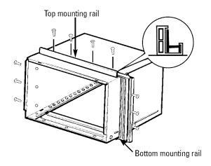
Insert the frames for the accordion panels into the top and bottom mounting rails. Attach the accordion panels to the side of the case using 6 type A screws.
