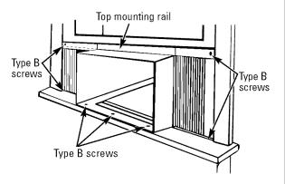
Extend the left and right accordion panels to the vertical window sashes and attach with 4 type B screws.
