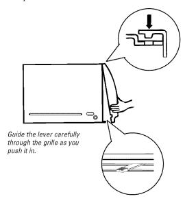
Secure the front grille to the case by replacing the screw removed in Step 3. If a screw was not removed in Step 3, secure the grille with a type A screw for models with a raise-up inlet grille or a type D screw for models with a slide-out filter.
