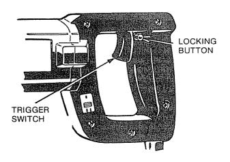
The Dual Speed Reciprocating Saw offers a choice of speeds for greatly improved cutting rates in various materials. Note that the High-Speed setting is more efficient in softer materials such as wood, while the Low-Speed is best for cutting metals
