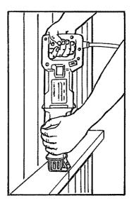
**CAUTION:** When sawing into walls, floors or wherever "live" electrical wires may be encountered, DO NOT TOUCH ANY METAL PARTS OF THE TOOL! Hold the tool only by the plastic handle and housing to prevent electric shock if you saw into a "live" wire.
