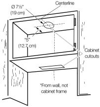
Style 4 - Cut Openings for 7" (17.8 cm) Round Vent to Round Vent Transition
