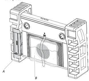
A. 31/4" x 10" (8.3 x 25.4 cm) rectangular vent damper B. 7" (17.8 cm) round vent mounting plate
