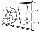
**3.**Remove the power supply knockout from the top or rear of the vent hood (depending on the incoming location of your home power supply cable) and install a UL listed or CSA approved ½" strain relief.
