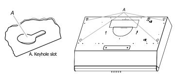
**3.**Use 1/8'' (3 mm) drill bit and drill 4 pilot holes as shown. NOTE: Make the drill holes on the thin area of the slot.
