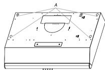
**2.**Use  $^{1/8}$ " (3 mm) drill bit and drill 4 pilot holes as shown. NOTE: Make the drill holes on the thin area of the slot.
