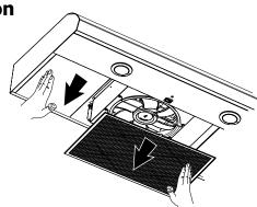
Remove the grease filter and the left side panel
