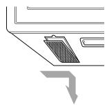
3. Remove charcoal filter by removing the vent grille mounting screws, tipping the grille forward and lifting out to remove. Open the microwave oven door. Then push the tab and lift the front of the filter up, and slide filter straight out.
