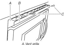
A. Vent grille B. Top louver C. Mounting screws
