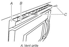
A. Vent grille B. Top louver C. Mounting screws 3. Tip the vent grille forward and down, then lift out to remove.
