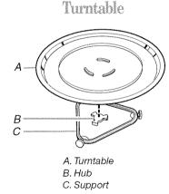
The turntable can rotate in either direction to help cook food more evenly. Do not operate the oven without having the turntable in place. See "Assistance or Service" to reorder any of the parts.
