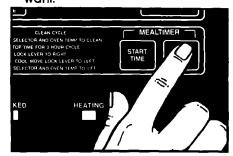
Touch the STOP TIME Pad. Then touch the Number Pads for the time you want baking to stop.
