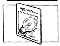
**3.** Remove the light bulb from its socket. Replace the bulb with a 40-watt appliance bulb.
