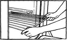
1. Position the rack(s) properly before turning on the oven. To change rack position, lift rack at front and pull out.
