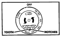
**3.** To lower the temperature, move the tooth a notch closer to LO. Each notch equals about 10°F (5°C).
