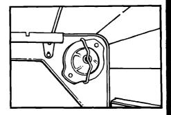
Replace the bulb cover and snap the wire holder in place. Turn the power back on at the main power supply.
