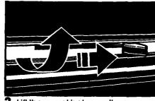
Lift the panel between the upper and lower oven doors. Move the Lock Lever all the way to the right.
