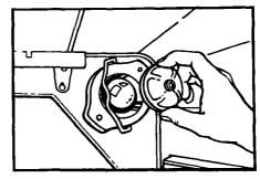
Remove the bulb cover in the back of the oven by pulling out and pushing the wire holder to the side.
