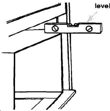
**3.** Lower window sash. Place level on the top edge of the cabinet. There should be a tilt to the outside of about one bubble. Place the level on the left side and check.
