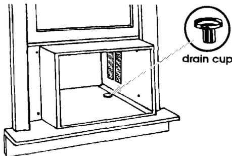
**4.** Place drain cup through hole in cabinet rail as shown.
