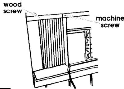
**7.** Pull out curtains and insert machine screws. Use a 2mm (3/32") drill bit to drill starter holes in the curtain housing. Fasten with wood screws.
