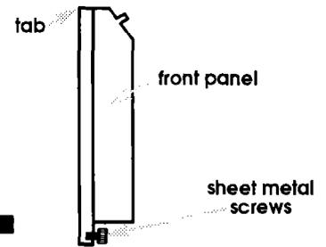
**9.** Unscrew sheet metal screws from front base flange. Insert tabs on the top edge of front panel into slots in the air conditioner cabinet. Use two sheet metal screws to attach the bottom of the front panel to the cabinet.
