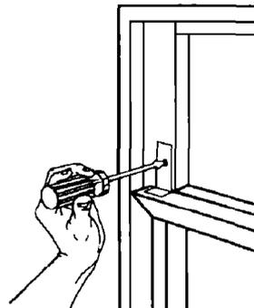
**8.** Insert window rail seal behind the top of the lower window sash and against the upper window sash. Use a 2mm (3/32") drill bit to drill a starter hole through the hole in the bracket.
