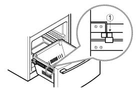
Remove the lower basket (2) by lifting basket from rail system.
