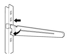
**NOTE:** Make sure that shelves are level from one side to the other. Failure to do so may result in the shelf falling or spilling food.
