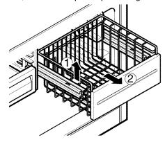
2. To Install, pull both rails out to full extension.
