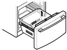
• Lift the top of door to unhook door supports from rail system. Lift door up to remove.
