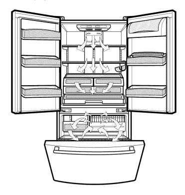
**Do not block any of cool air vents** with food packages. If the vents are blocked, airflow will be interrupted and temperature and moisture problems may occur.
