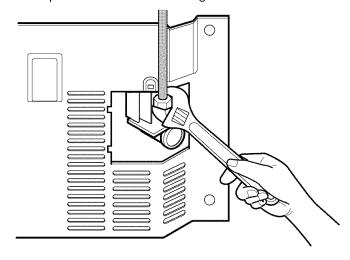
**5.** Bend the pipe to upwards and replace the cover into original position. And tighten the screw.
