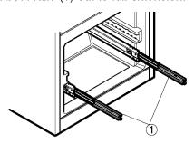
• Hook the door supports (2) into the rail tabs (3), as illustrated, and lower the door into final position.
