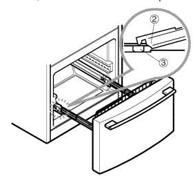
• With the drawer pulled out to full extension, insert the lower basket (4) in the rail assembly until it doesn't move forward.
