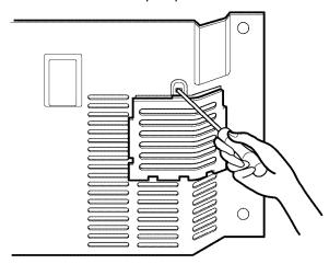
2. Lift off the cover by slightly pushing up.
